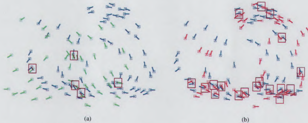
Fig. 3. Minutiae matching for (a) twin–nontwin (matching of Figs. 2(e) and (f), matching score = 3 on a scale of 0–999) and (b) twin–twin (matching of Figs. 2(d) and (e), matching score = 38 on a scale of 0–999). The “matched” minutiae pairs are shown by bounding boxes.
